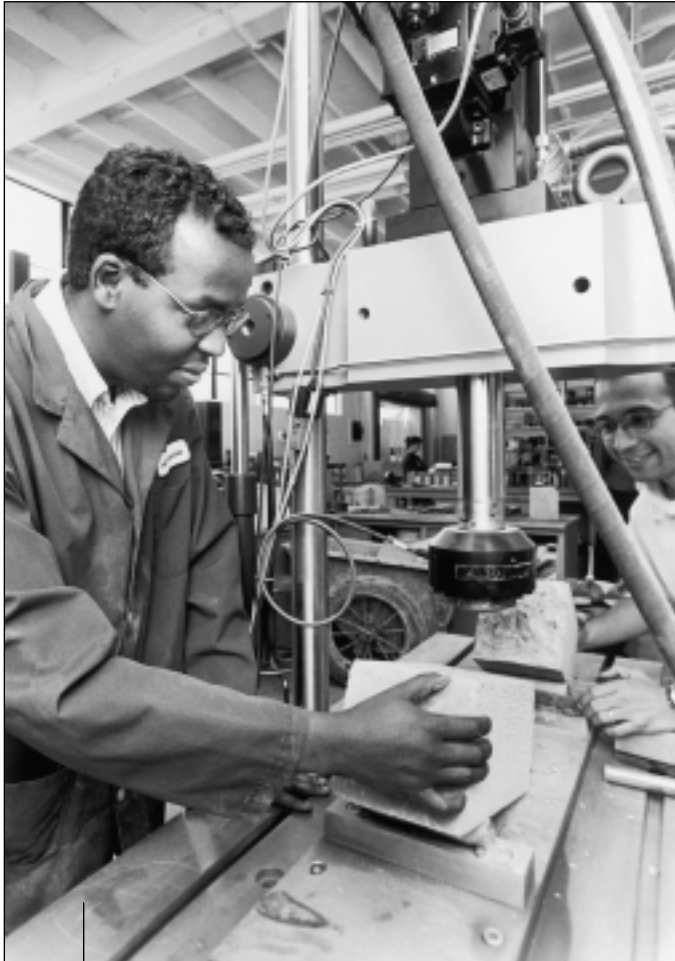
Abdikarim Ali (left) and Manuel Bejarano stress a concrete beam until it fails.
